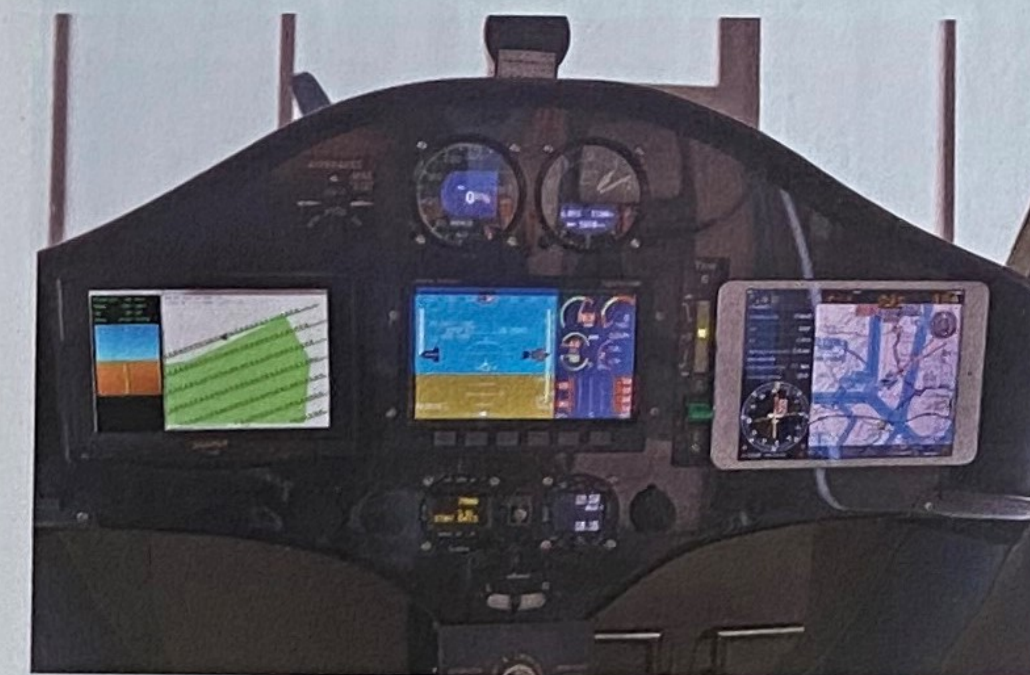
The Green Observer operates from the Chambley airfield in eastern France; the AirPhotoNav flight management system is mounted on the far left in the cockpit.
